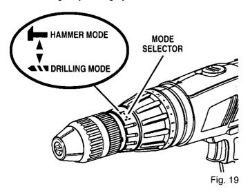
We recommend that you use carbide-tipped bits and select hammer mode when drilling in hard materials such as brick, tile, concrete, etc.
